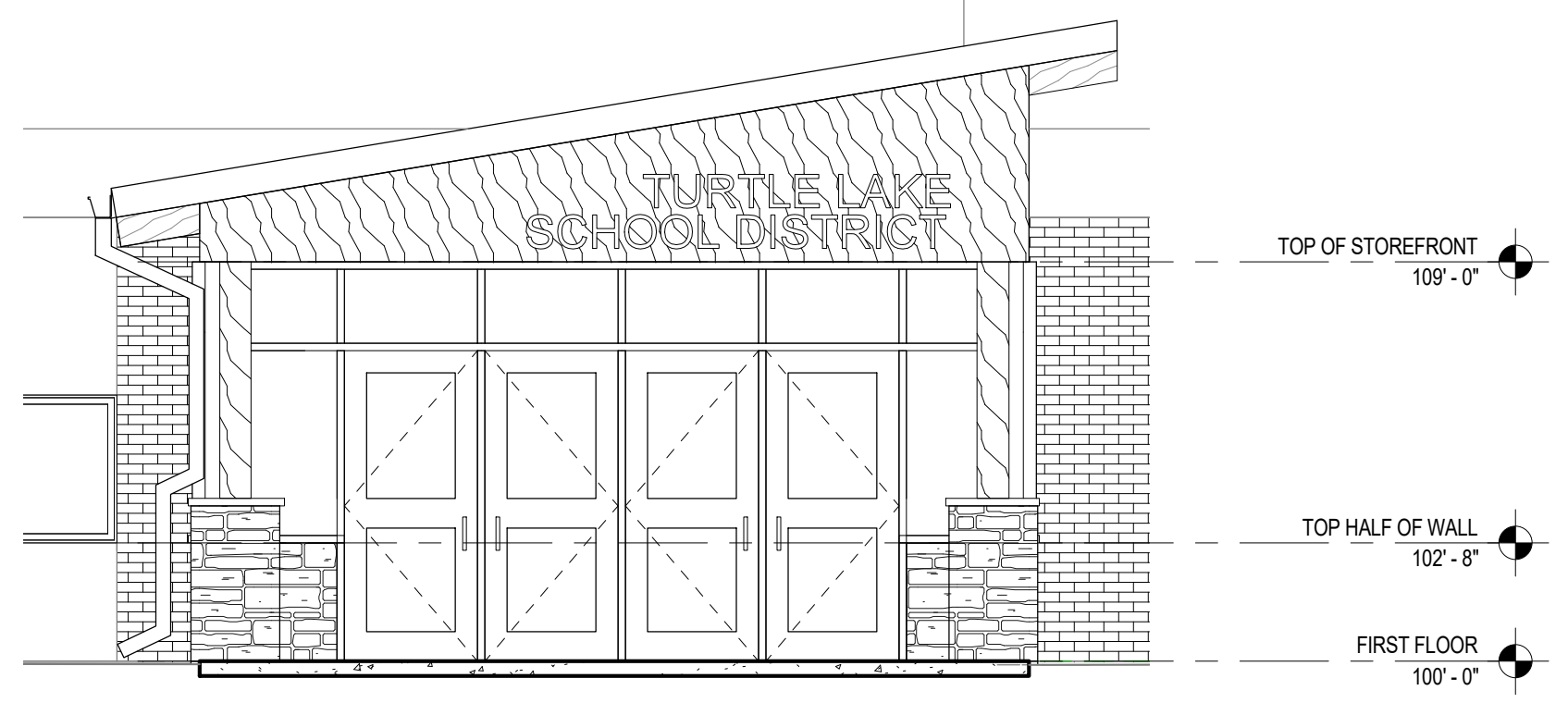
5 ENTRY - FRONT ELEVATION 1/4" = 1'-0"
